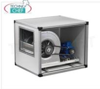
**ASPIRATORE CASSONATO con VENTILATORE CENTRIFUGO a TRASMISSIONE con CINGHIE e PULEGGE, pannellature INOX, 2 VELOCITA', portata max 10000/6690 m/cubi/ora, giri 900/602, db 77/64, V.380/3, Kw.4,2/1,4, Peso 117 Kg, dim.mm.1200x1000x1000h**
