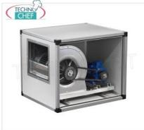
**ASPIRATORE CASSONATO con VENTILATORE CENTRIFUGO a TRASMISSIONE con CINGHIE e PULEGGE, pannellature INOX, 2 VELOCITA', portata max 15000/10034 m/cubi/ora, giri 700/468, db 73/64, V.380/3, Kw.4,2/1,4, Peso 118 Kg, dim.mm.1200x1000x1000h**
