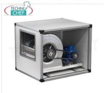
**ASPIRATORE CASSONATO con VENTILATORE CENTRIFUGO a TRASMISSIONE con CINGHIE e PULEGGE, pannellature INOX, 2 VELOCITA', portata max 12000/8028 m/cubi/ora, giri 870/582, db 78/66, V.380/3, Kw.4,2/1,4, Peso 117 Kg, dim.mm.1200x1000x1000h**
