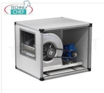
**ASPIRATORE CASSONATO con VENTILATORE CENTRIFUGO a TRASMISSIONE con CINGHIE e PULEGGE, pannellature INOX, 2 VELOCITA', portata max 12000/8028 m/cubi/ora, giri 780/522, db 76/64, V.380/3, Kw.4,2/1,4, Peso 117 Kg, dim.mm.1200x1000x1000h**
