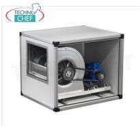
**ASPIRATORE CASSONATO con VENTILATORE CENTRIFUGO a TRASMISSIONE con CINGHIE e PULEGGE, pannellature INOX, 2 VELOCITA', portata max 13000/8757 m/cubi/ora, giri 730/492, db 70/61, V.380/3, Kw.3,0/0,9, Peso 117 Kg, dim.mm.1200x1000x1000h**
