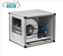
**ASPIRATORE CASSONATO con VENTILATORE CENTRIFUGO a TRASMISSIONE con CINGHIE e PULEGGE, pannellature INOX, 2 VELOCITA', portata max 11000/7410 m/cubi/ora, giri 770/519, db 69/59, V.380/3, Kw.3,0/0,9, Peso 117 Kg, dim.mm.1200x1000x1000h**
